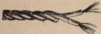
FIG. 252.—A twisted pair of insulated wires, forming two sides of a single circuit, as in telephone cables.
